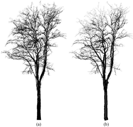
Fig. 3. Example (a) TLS point cloud from a 120-cm-diameter Liriodendron tulipifera and the resulting (b) 3-D TLS model.
